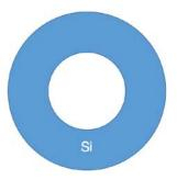
b. A long cylindrical Si tube of inner radius 3  $\mu$ m and outer radius 4  $\mu$ m is placed in an oxidation chamber (shown above). Assume oxidation proceeds identically from the outside and the inside of the tube. At what distance from the center will the two Si/SiO<sub>2</sub> interfaces meet? What if the inner radius is 1  $\mu$ m instead?
